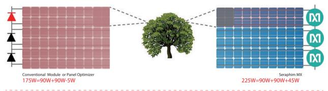
Seraphim MX reduces the shading effect significantly, prevents hot-spot formation, and eliminates diode failures. In the meantime, it will lower Operation and Maintenance costs.
