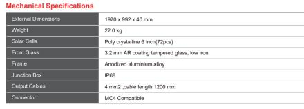
STC: Irradiance 1000 W/m², module temperature 25°C, AM=1.5 NCCT: Irradiance 800 W/m², ambient temperature 20°C, wind speed :1m/s Specifications are subject to change without further notification.
